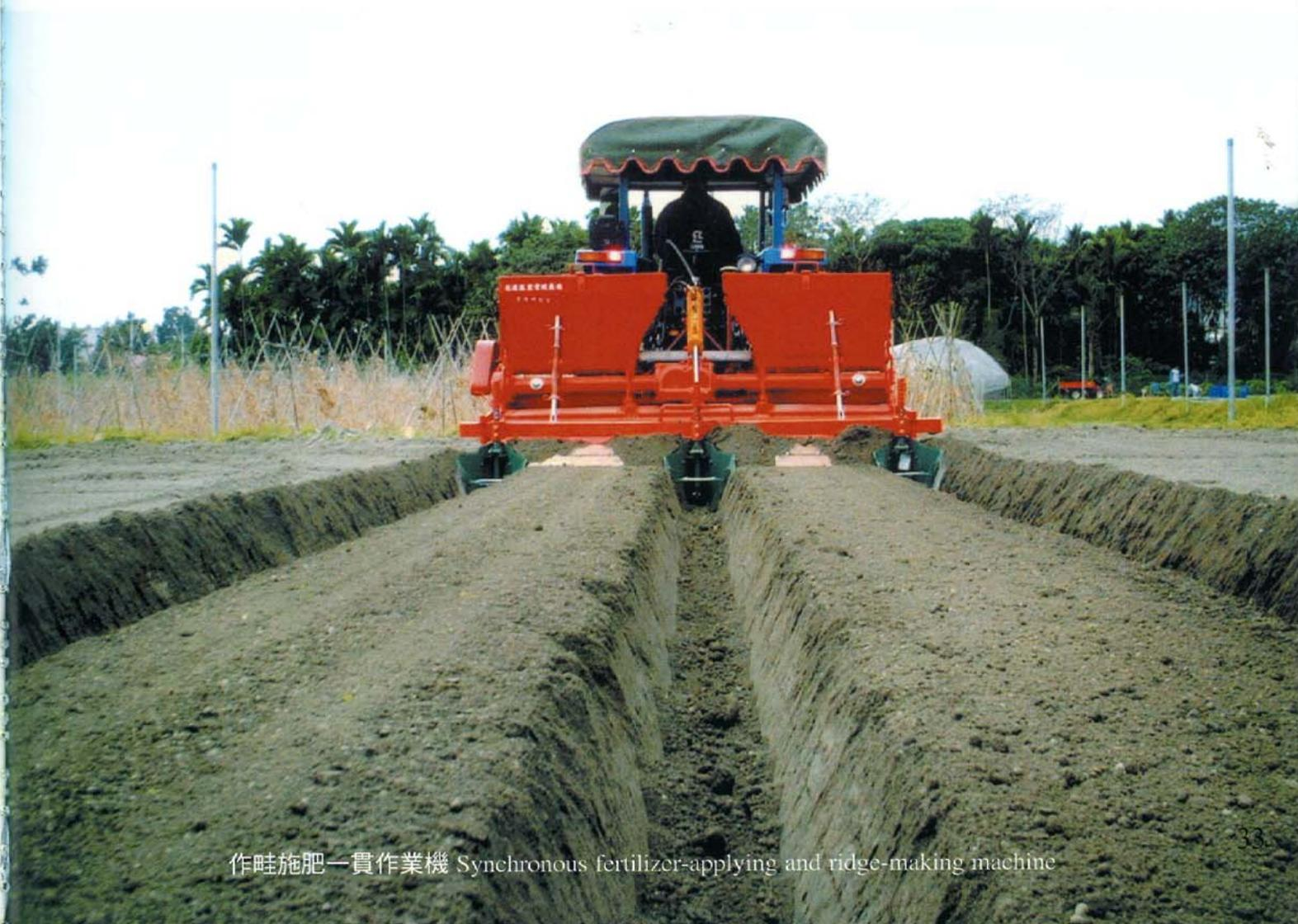
作畦施肥一貫作業機 Synchronous fertilizer-applying and ridge-making machine
