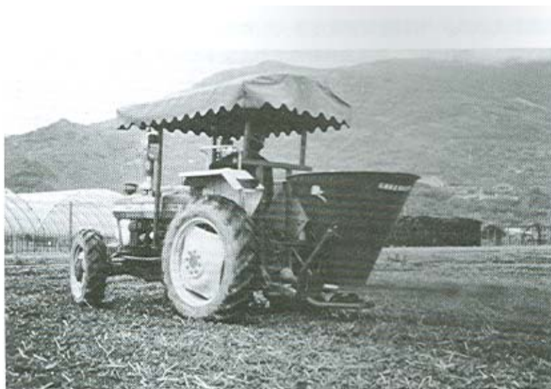
圖一、開發完成 0.5m 3 之綜合型肥料撒佈機 Fig.1 Multifunctional manure spreading machine with 0.5m 3 capacity.
