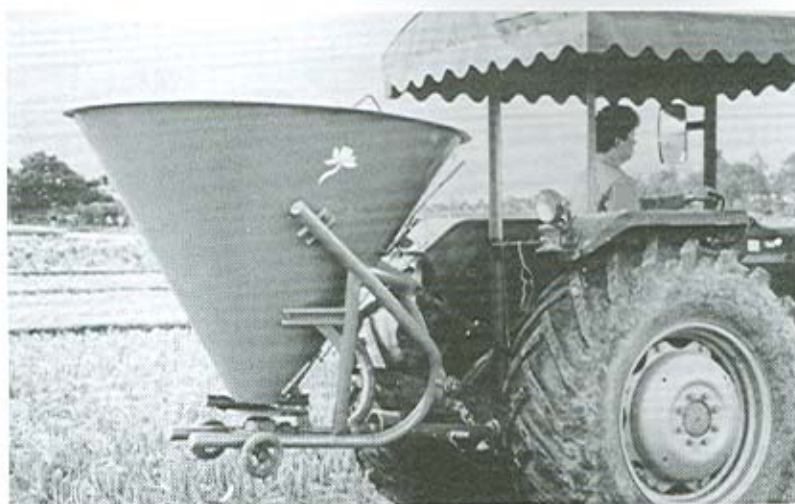
圖二、研製完成 1.0 m 3 之綜合型肥料撒佈機外觀 Fig.2 Multifunctional manure spreading machine with 1.0 m 3 capacity.
